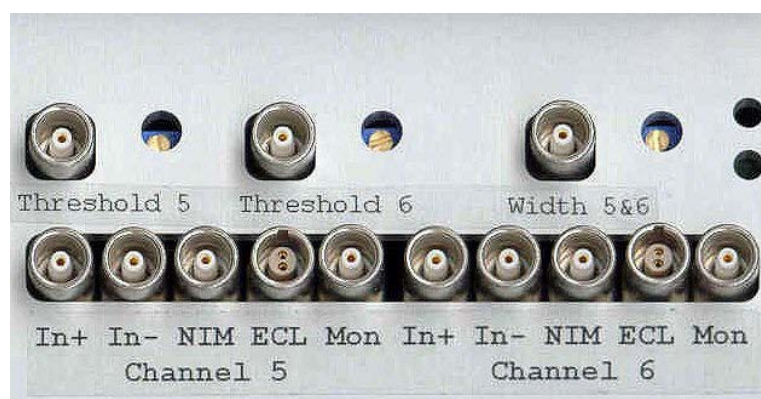
Figure 3.7: inputs, outputs and controls of the ATR19 (here version -6/8) for each internal DLATR board
